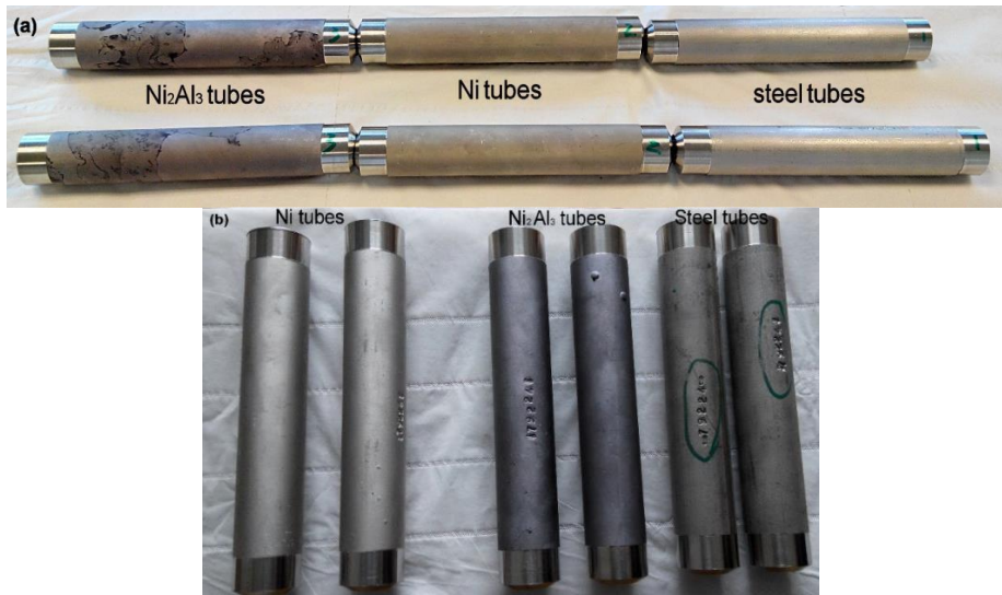
Figure 7. Appearance of the first set of test tubes for (a) Esshete 1250 and (b) TP347H.
