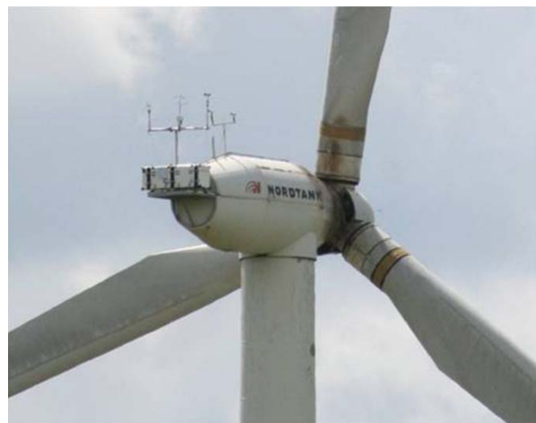
Figure 23: LiDAR mounted on the rear of the NTK 500kW turbine at the DTU Risø test site.
