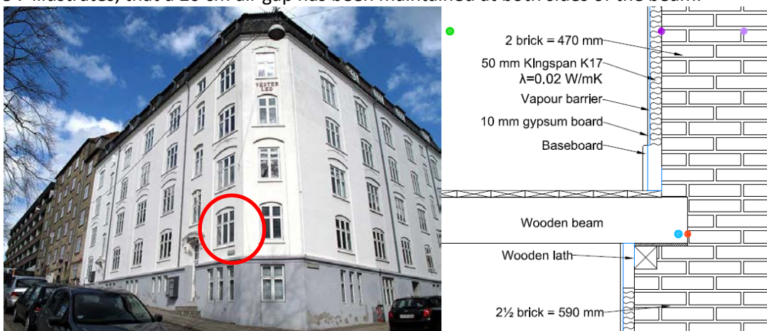
Figure 7: Mønsgade and indication of wall placement (left) and construction with sensor placement (right)
