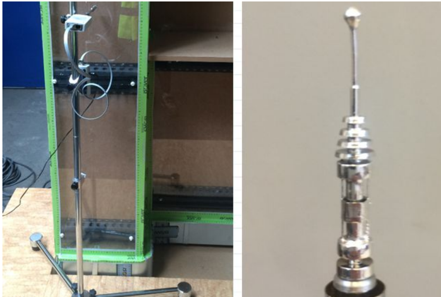
Figure 51: Set-up of the anemometer (left), sensor of the anemometer (right)
