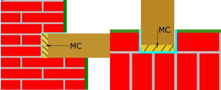
Figure 29: Location at beam where MC is investigated, M4 (left) and M5 (right)
