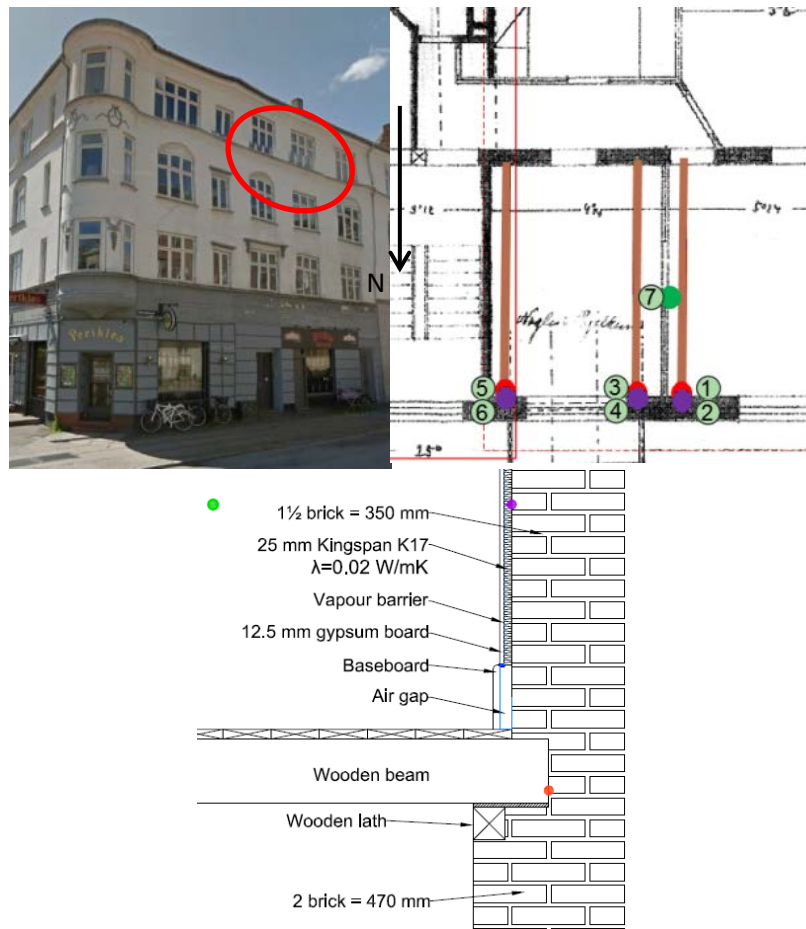
Figure 4: Kildevældsgade and indication of wall placement (left), sensor placement on floor plan (middle) and construction with sensor placement (right)
