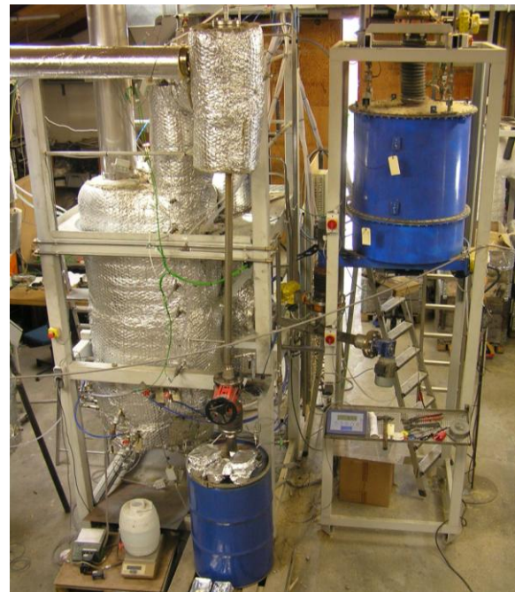
Figure 3: 100 kW LT-CFB gasifier at DTU. The gasifier is the parts in alu-folio, while the blue barrels are the (elevated) fuel bin and the bin for ash separated by the secondary cyclone.
