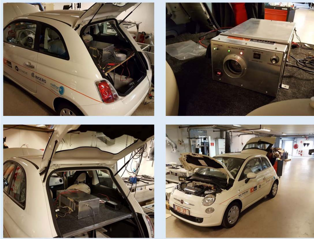
Figure 1 Installation of ENTIFVIC EV in Fiat 500 EV.
