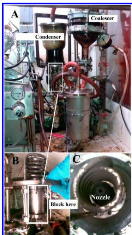
Figure 5. The block at nozzle (A: bio-oil condensing system, B: nozzle in front view, C: nozzle in top view).
