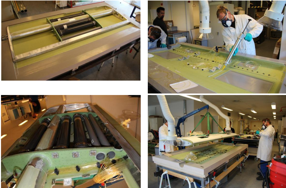
Figure 26 The manufacturing of the 2m long blade section in the fiberlab workshop at DTU.
