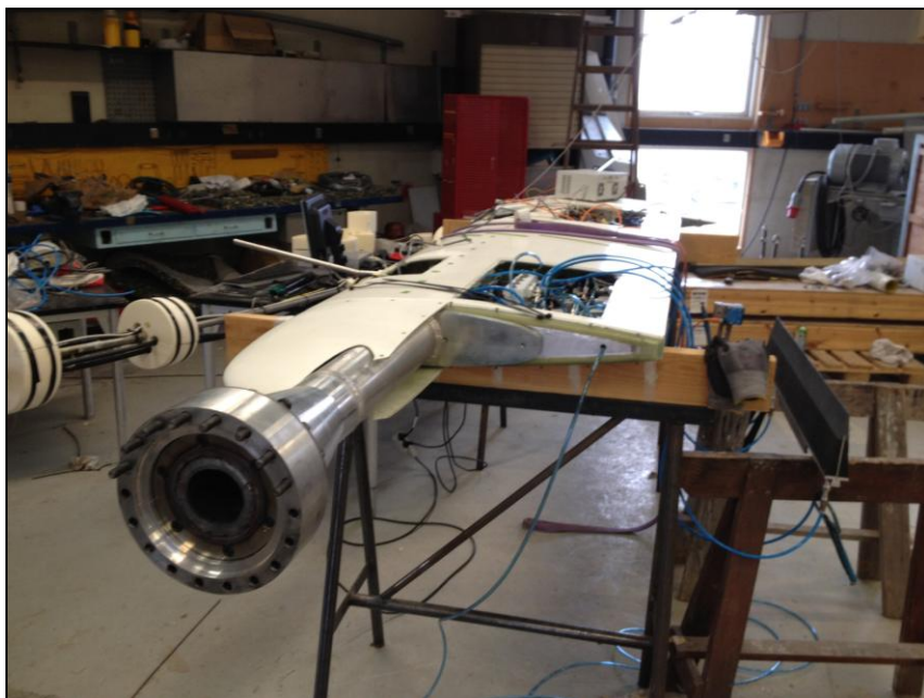
Figure 27 Assembling the blade section with part of the boom.
