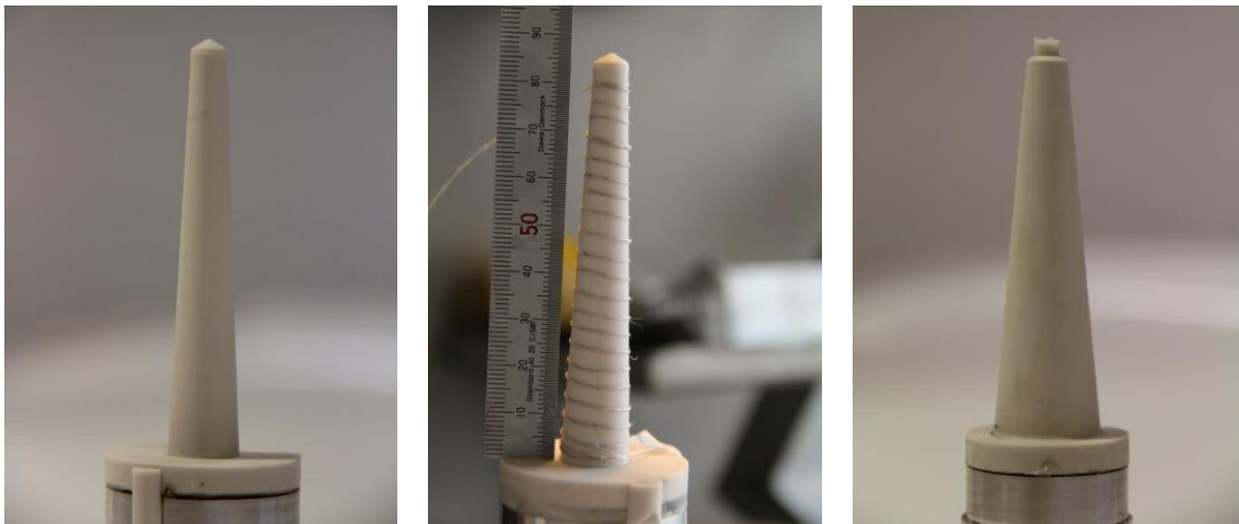
Figure 15 Concept for manufacture of non-metallic springs. Step1: Casting of inner liner, step 2: Winding of non-metallic spring element and step 3: Fixation of reinforcement by second casting.
