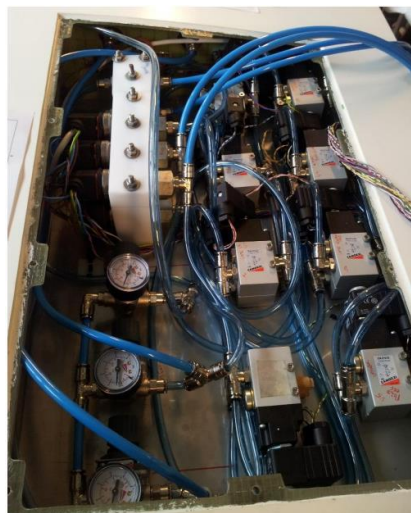
Figure 19 To the left is shown a sketch of the blade section for the rotating test rig and to the right the pneumatic control system is installed in the blade section.
