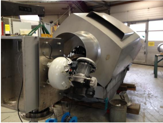
Figure 28 The compressor for the pneumatic activation of the flap was mounted on the hub as seen on the photo to the left. To the right the slip rings are seen which were both transmitting the measurement signals as well as supplying electrical power to the compressor
