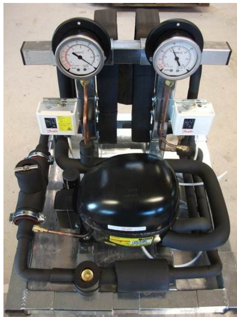
Figure 8: Heat pump prototype used for laboratory test
