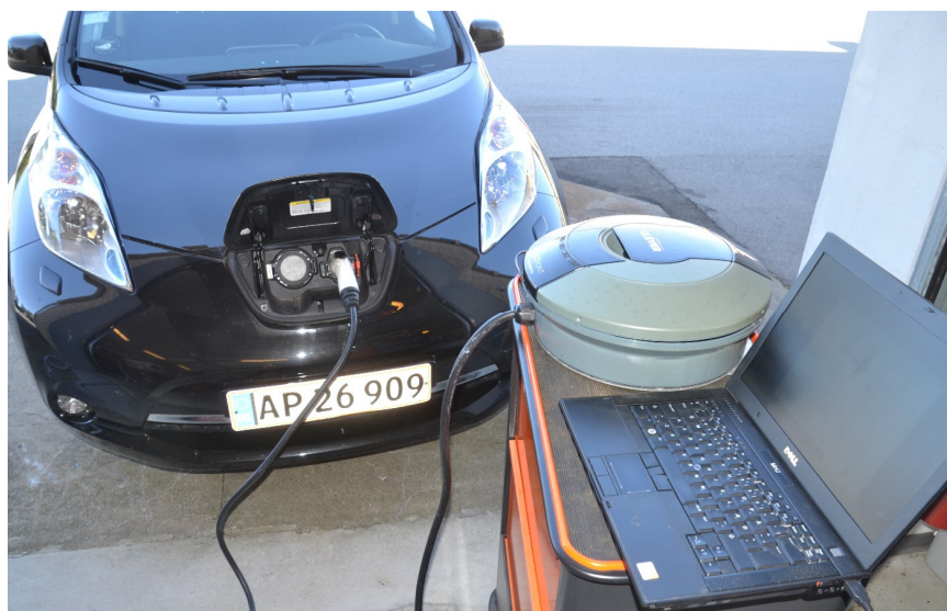
Figur 7 EV test charge using EV Home charger made “SG Ready” via remote control of charge current from Labview SW also emulating control from SG Ready inputs
