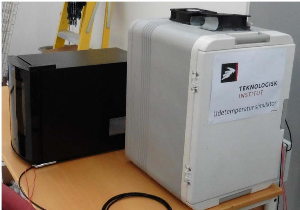
Figure 22 Two remotely temperature controlled cabinets for simulating house in-door temperature (left) and out-door temperature (right) used for manipulating the heat pump original sensors.
