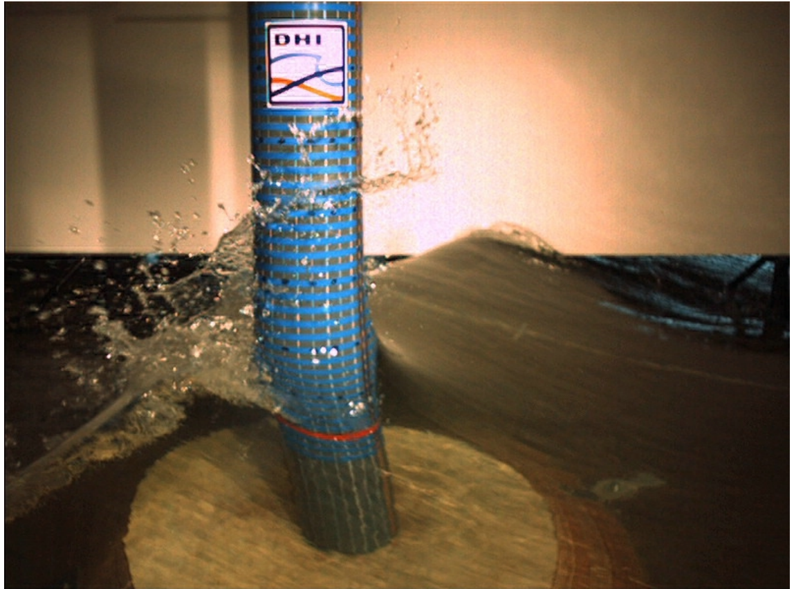
Fig 3.3 Run-up in the physical model. A plywood base with the envelope of a typical scour protection is applied to study the effect of the scour protection.
