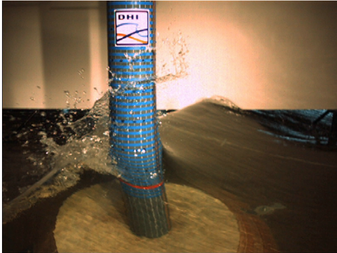
Figure 9 Wave run-up on a pile. It is seen that the front of the run-up is thicker than the rest of the run-up. The front is approximately 40cm above SWL (red line) (the blue/grey lines are 1cm each and there are 10cm between the blue lines with black dots).
