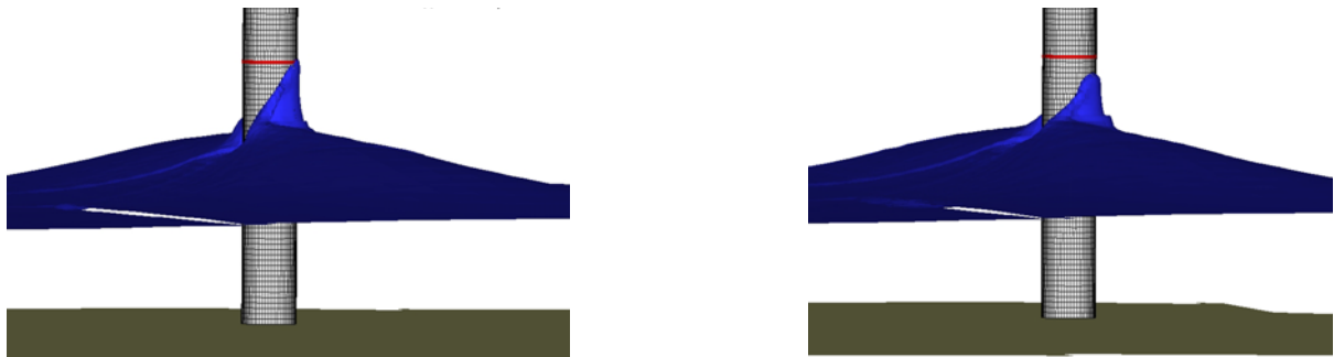
Figure 7 Wave run-up for two different grid resolutions. The figure to the left shows the run-up for a grid resolution of 0.60x0.78x1.58cm, while the figure to the right shows the run-up for a grid resolution of 1.37x0.78x1.58cm
