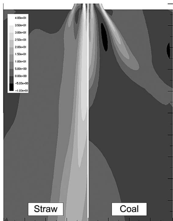
Fig. 8. Contours of axial velocity [m/s] on horizontal half plane. Grid: 4 \times 10 m.
