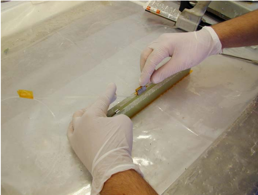
Figure 5. Showing the insertion of a fibre optic microbend transducer into the adhesive bondline during composite DCB specimen fabrication
