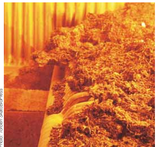
Combustion of straw on vibrating grate. Today, grate-firing is the most widespread technology for combustion of biomass in power plant boilers.
