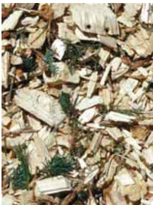
There are different types of wood chips. The length may vary between 5 and 50 millimetres and wood chips may contain small twigs.
