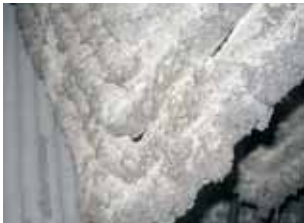
Deposits on superheater tubes at a straw-fired power plant.
