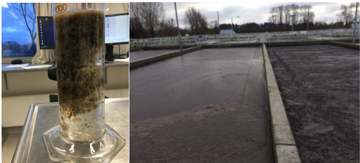
Figure 7: Left: 25-01-2018, sludge floats to the surface after 45 min. in the laboratorie Right: 26-01-2018, the surface if the clarifiers are covered with sludge
