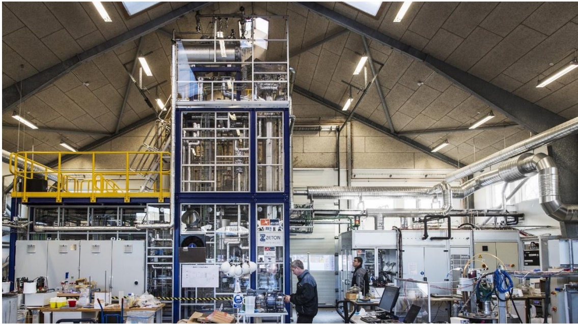
Figure 3-2: The pilot plant at AU Foulum site. The tall reactor and steam drum makes the pilot plant reach the rooftop.
