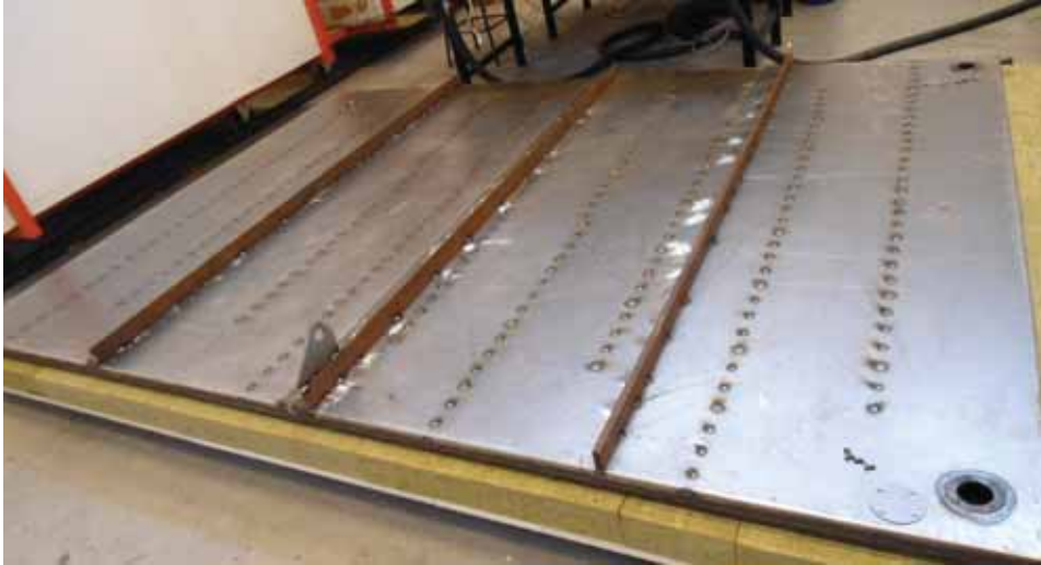
Fig. 6. Photos of the second heat storage module with two holes used to fill in the salt water mixture.
