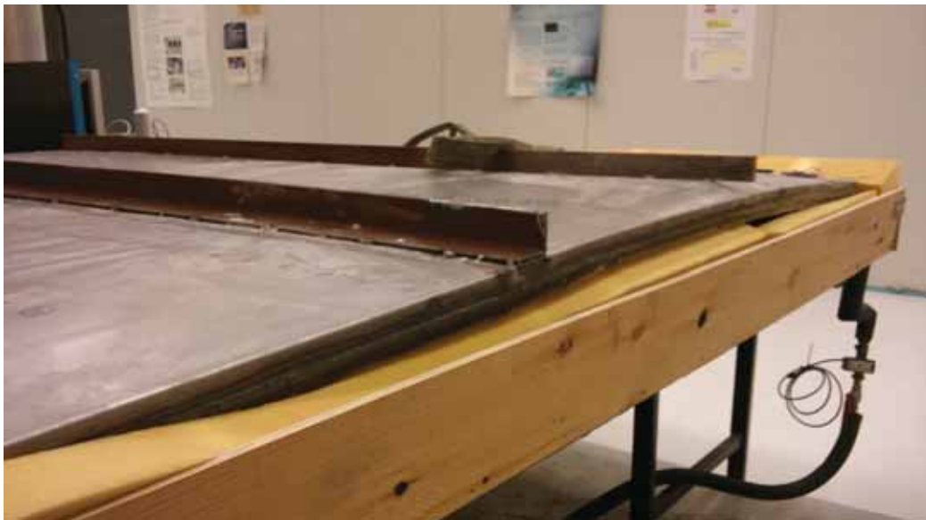
Figure 12: Photo of the damaged second heat storage module.
