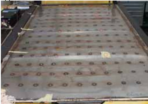
Fig. 1: Photo of the PCM heat storage test module with plate heat exchangers at the top and the bottom.
