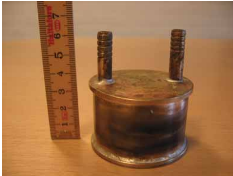
Fig. 5: Brass tank with CO 2 used for starting the solidification.
