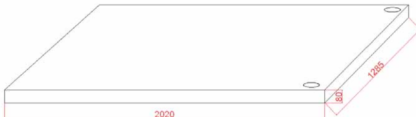
Fig. 1. Principle sketch of the first heat storage module with two holes used to fill in the salt water mixture.
