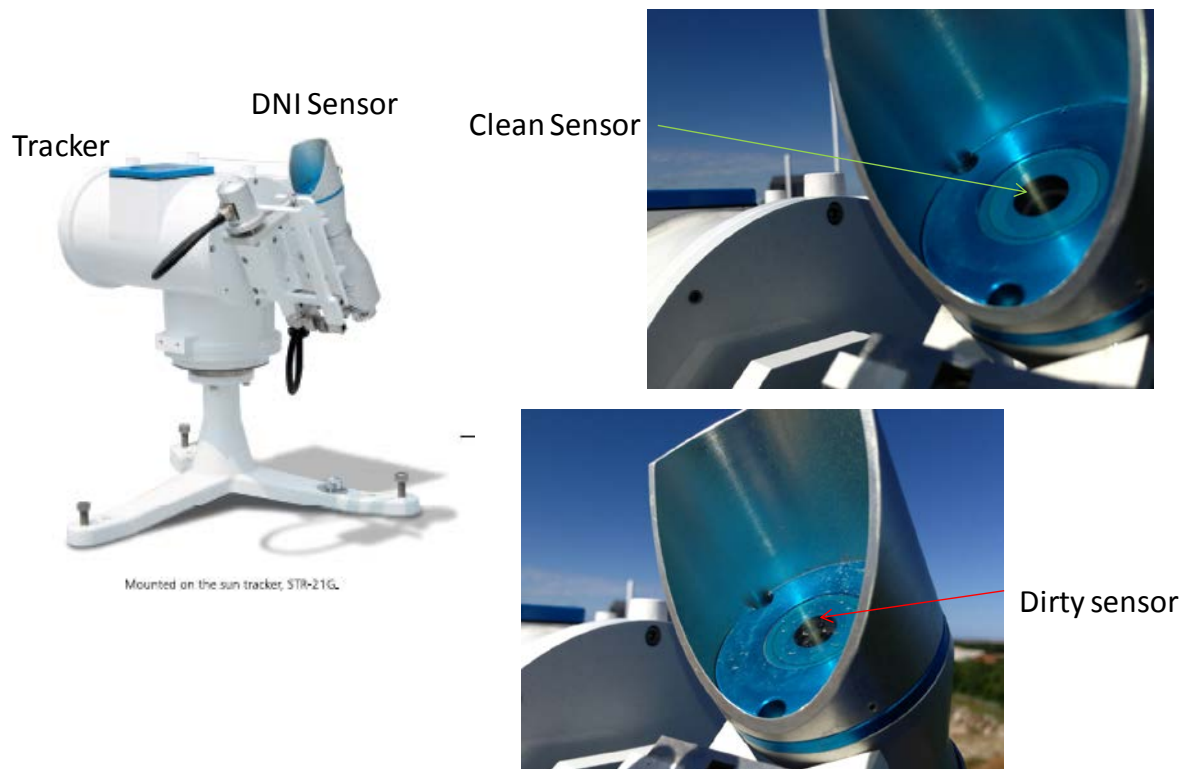
Figure 3. Pyrheliometer for measurement of direct radiation. A problem with soiling of the sensor was identified and regular cleaning was applied to have accurate longterm data. Construction work nearby the plant probably enhanced this problem significantly. On other pyrheliometer instruments the rain shelter is not there, leading to self cleaning in the Nordic climate conditions.
