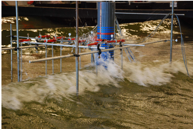
Figure 72: Breaking wave impact at scale 1:36.6.
