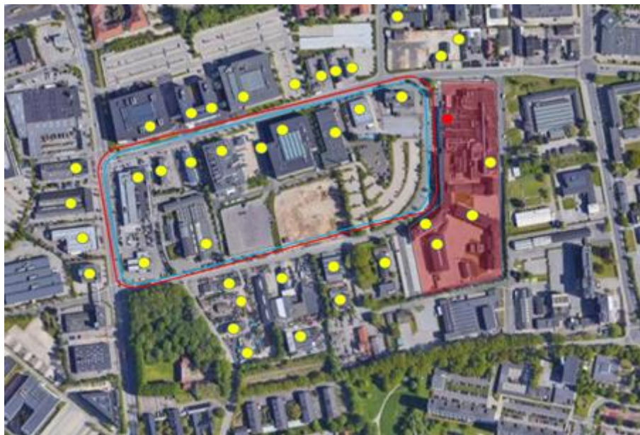
Figure 3: Commercial area in northern Copenhagen – the red point represents the excess heat available, while the yellow ones the consumers for the specific area
