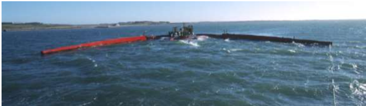
Figure 4.2: The 58 m wide prototype scale 1:4.5 of a 4 MW device in Nissum Bredning 2003 - 2010 showing the two reflectors that focus waves towards the ramp and the reservoir that stores overtopping water [2]
