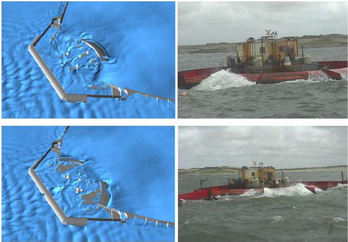
Figure 5.6 Comparison of CFD simulations with Nissum Bredning web-cam pictures. The overtopping patterns are quite alike and the numerical results are also in line with model tests in scale 1:50 [66]
